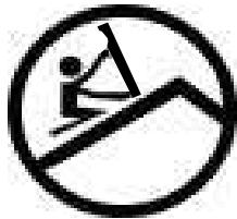
EternaTile installed from the bottom
